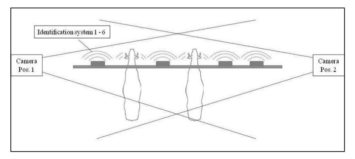
Figure 4. Position of the two cameras
