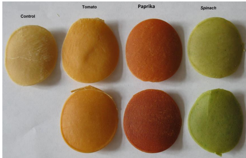
The coloured pastas after 30 days stored in dark Top: 5 g additives, bottom: 10 g additives
